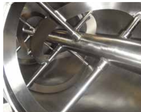
304L / 316L stainless-steel internal polishing
